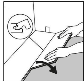
Place the first plank of the new row with the tongue side at an angle against the groove side of the plank in the previous row. Press forward and lay it flat at the same time.
