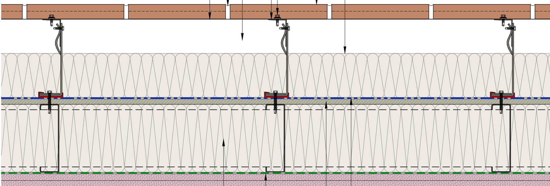
SFS with full fill insulation between studs.
