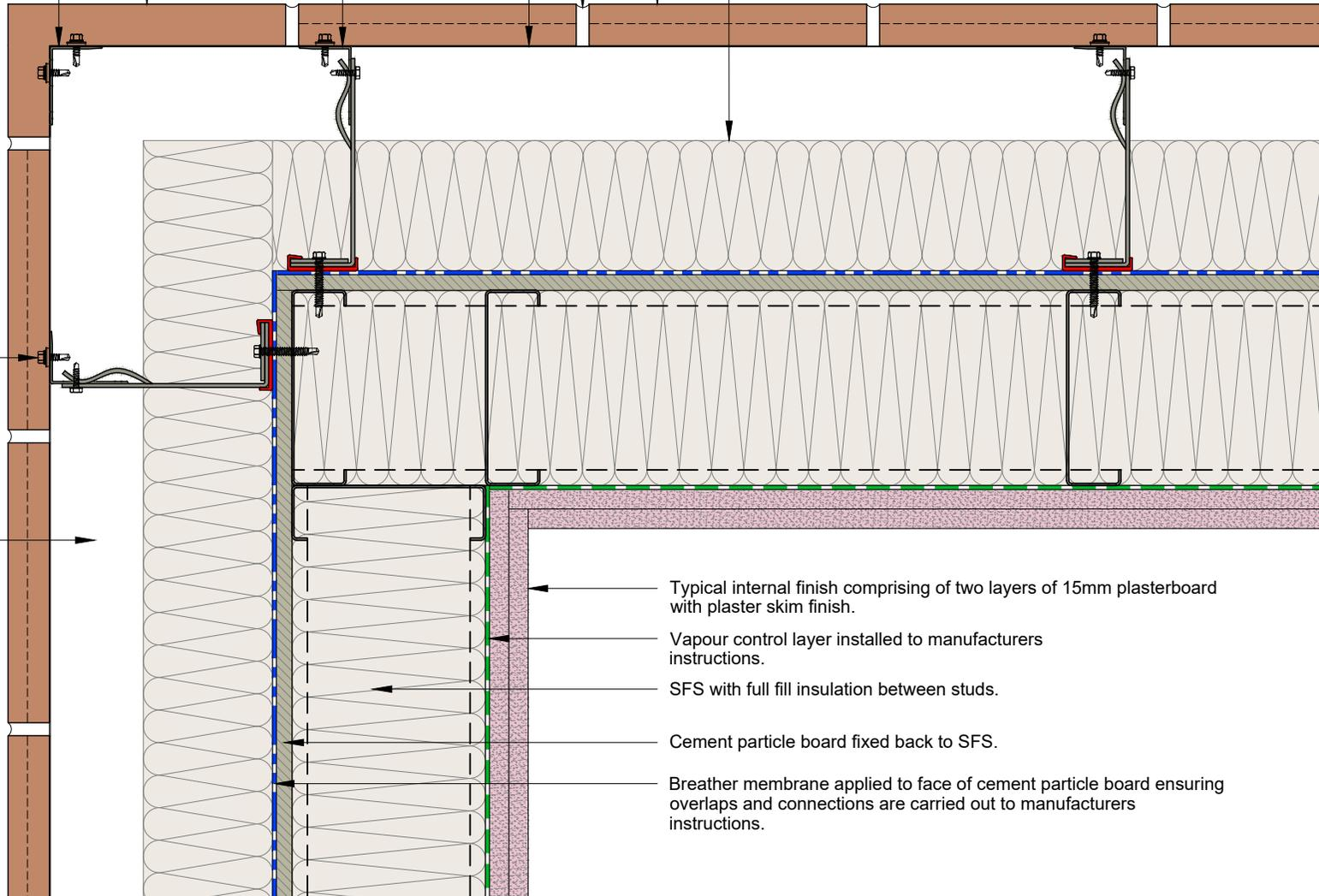
Typical internal finish comprising of two layers of 15mm plasterboard with plaster skim finish.
