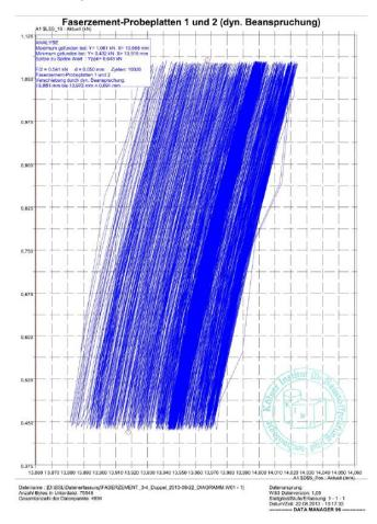
The displacement before and after the pulsating loading is 0,091 mm.
