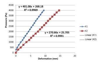
The load at which the test specimen fails is 4350 Pa, at which moment a panel breaks in a corner.
