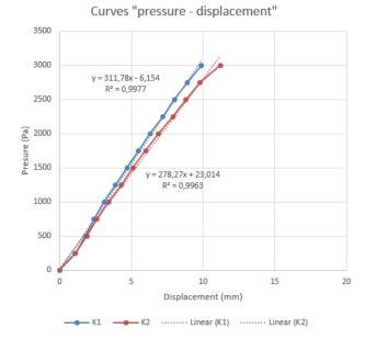
The load at which the test specimen fails is 4867 Pa, at which moment a panel breaks in all four corners.
